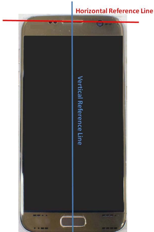
SAR Test Setup Photo 7: Horizontal and Vertical Reference Lines
