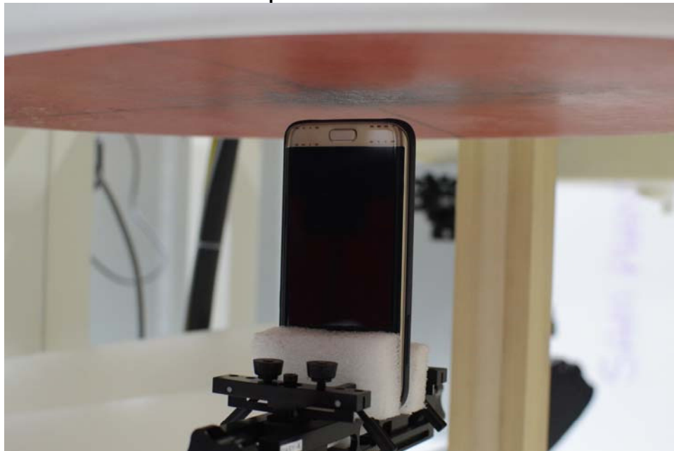
SAR Test Setup Photo 6: Bottom Edge at 1.0cm
