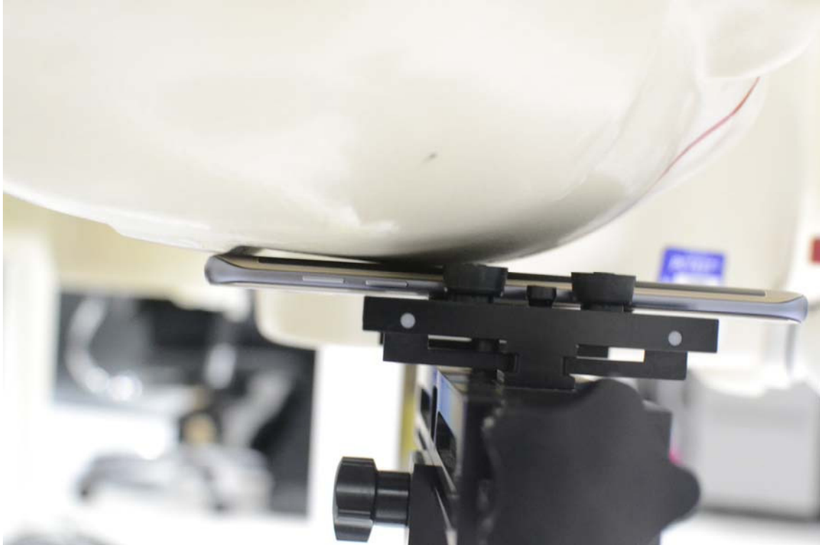
SAR Test Setup Photo 1: Right Cheek
