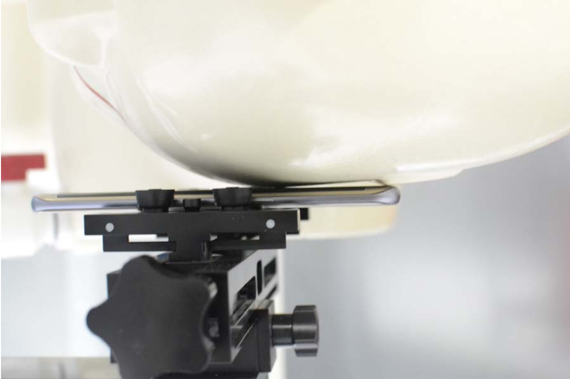
SAR Test Setup Photo 3: Left Cheek
