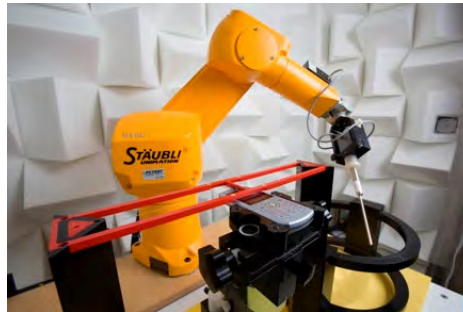
Figure 5-3 SPEAG Robotic System
