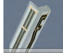
Figure 5-1 E-field Free-space Probe
