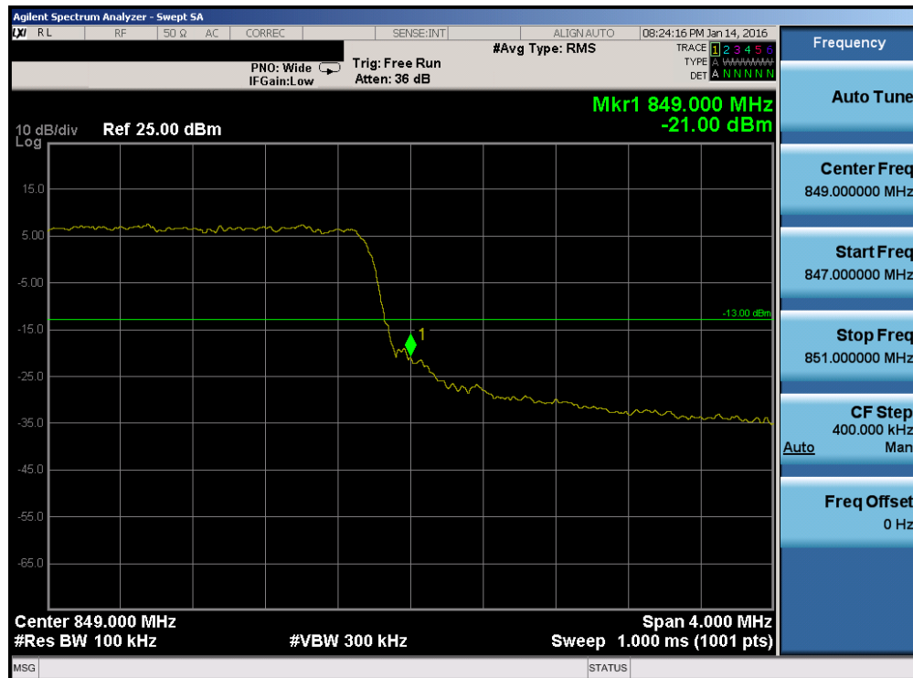
Plot 7-152. Upper Band Edge Plot (Band 5 – 5.0MHz QPSK – RB Size 25)
