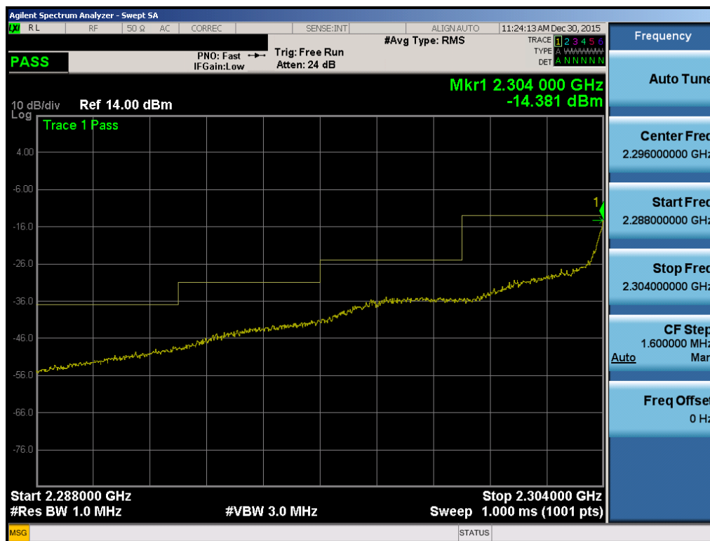
Plot 7-204. Lower Extended Band Edge Plot (Band 30 – 5.0MHz QPSK – RB Size 25)
