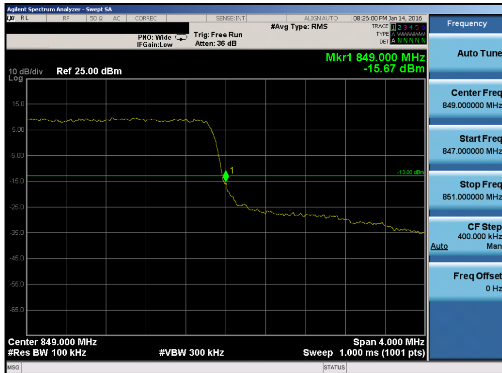
Plot 7-150. Upper Band Edge Plot (Band 5 – 3.0MHz QPSK – RB Size 15)
