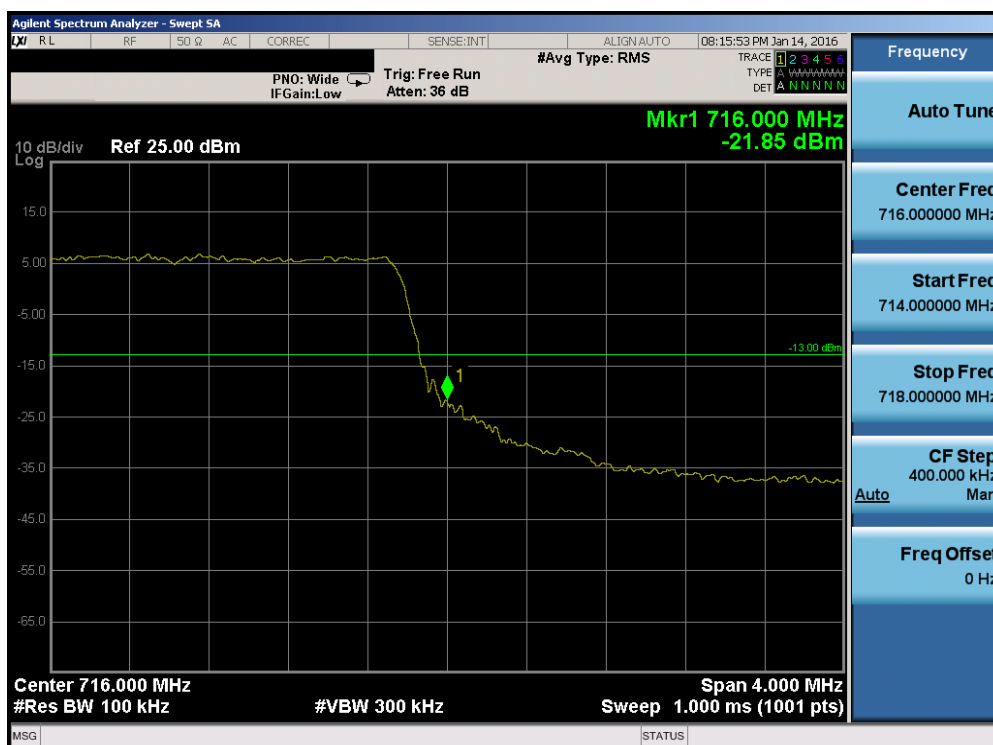
Plot 7-136. Upper Band Edge Plot (Band 17 – 5.0MHz QPSK – RB Size 25)
