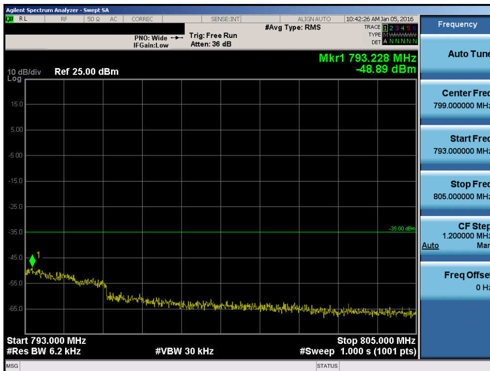
Plot 7-146. Upper Emission Mask Edge Plot (Band 13 – 10.0MHz QPSK – RB Size 50)
