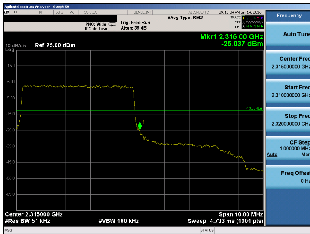
Plot 7-205. Upper Band Edge Plot (Band 30 – 5.0MHz QPSK – RB Size 25)
