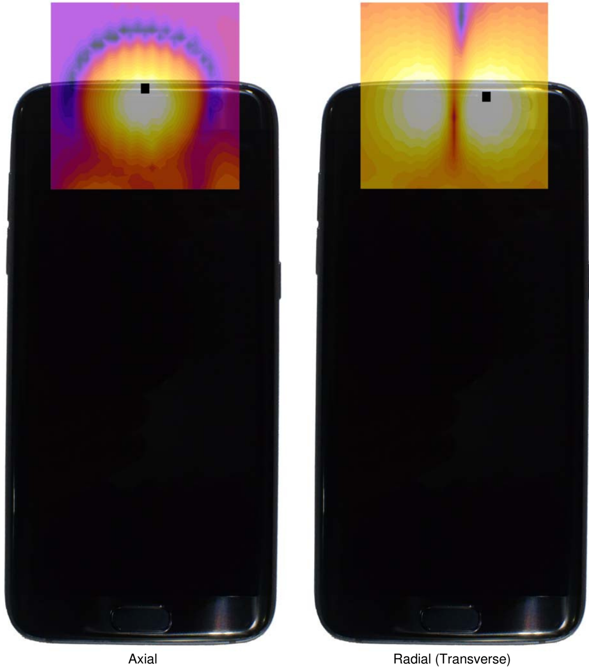
Figure 15-3 T-Coil Scan Overlay Magnetic Field Distributions
