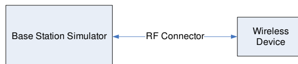
Figure 9-B Power Measurement Setup
