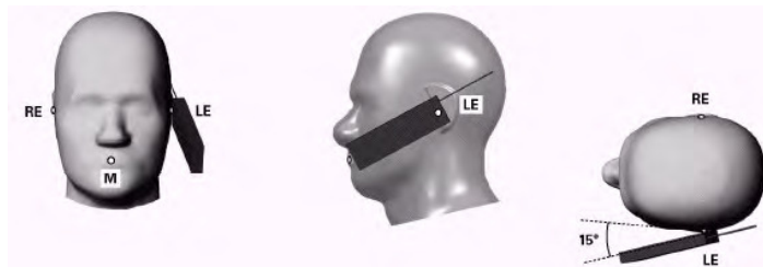
Figure 6-B Front, Side and Top View of Ear/15° Tilt Position
