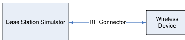
Figure 9-A Power Measurement Setup
