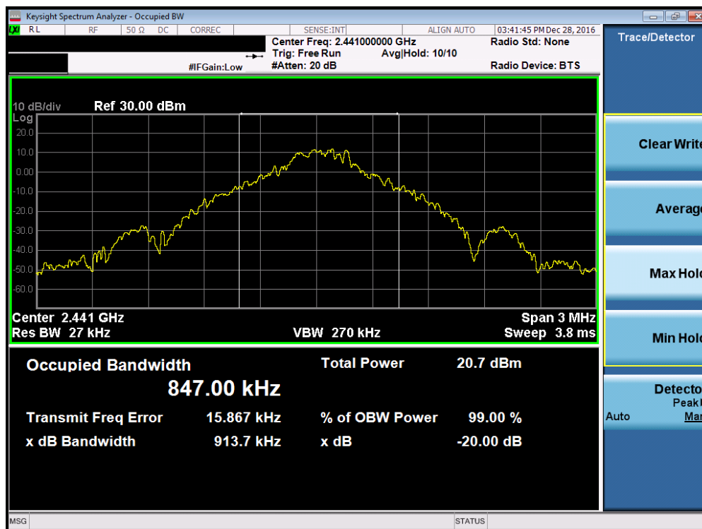
Plot 7-2. 20dB Bandwidth Plot (Bluetooth, 1Mbps – Ch. 39)
