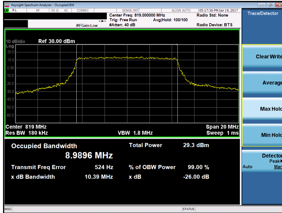
Plot 7-21. Occupied Bandwidth Plot (10MHz 64-QAM – RB Size 50)
