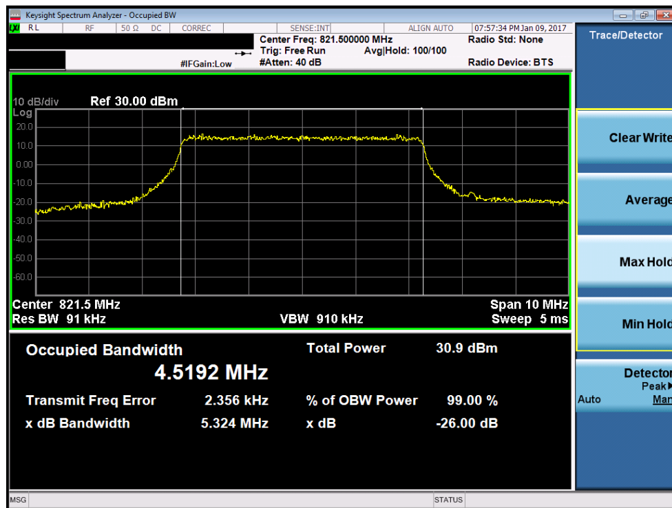
Plot 7-16. Occupied Bandwidth Plot (5MHz QPSK – RB Size 25– High Channel)
