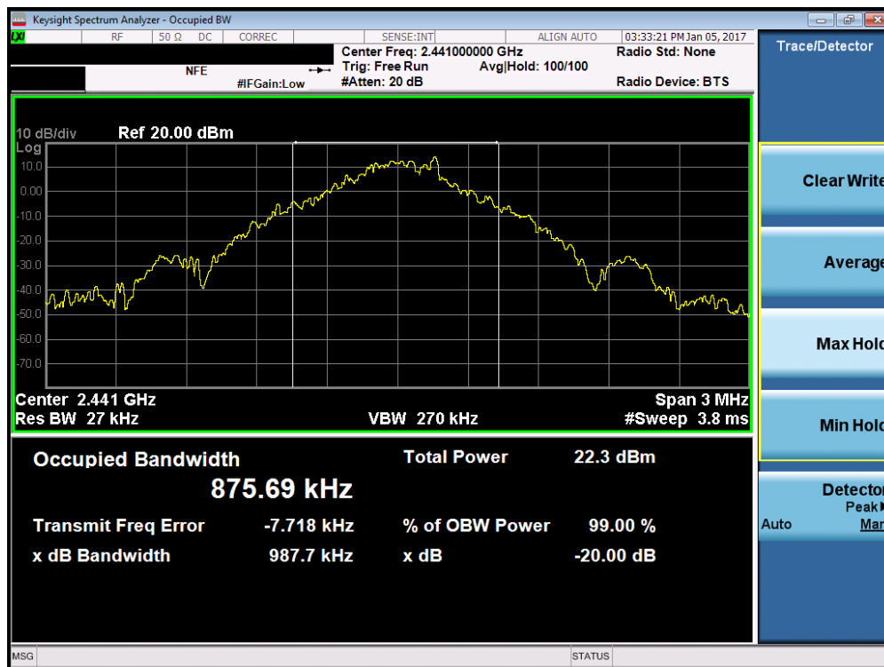
Plot 7-2. 20dB Bandwidth Plot (Bluetooth, 1Mbps – Ch. 39)
