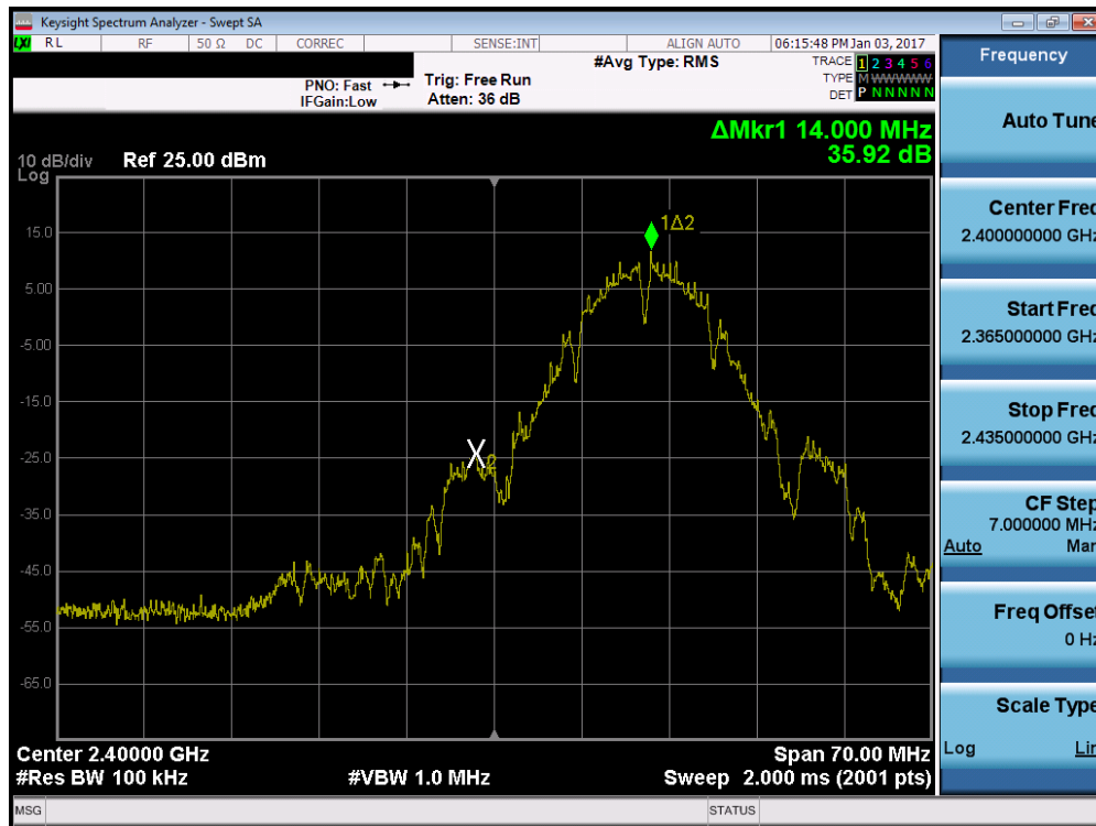
Plot 7-37. Band Edge Plot (802.11b – Ch. 1)
