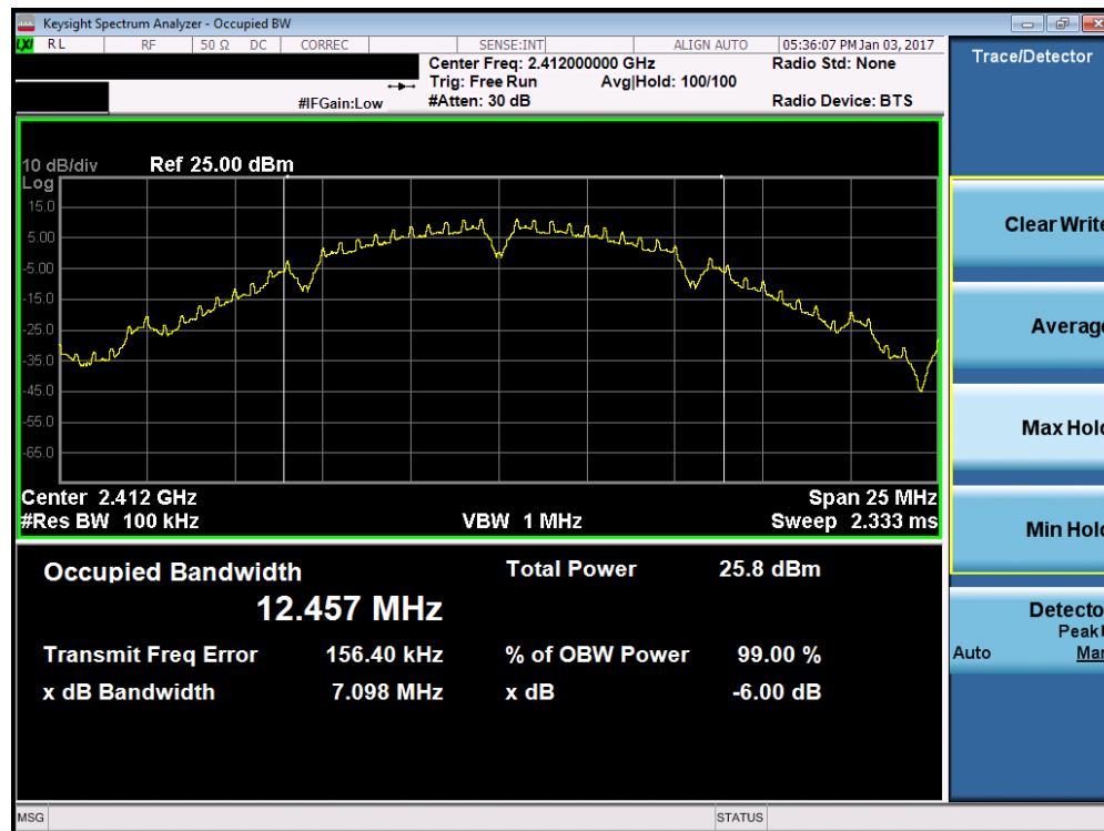
Plot 7-10. 6dB Bandwidth Plot (802.11b – Ch. 1)
