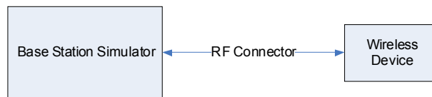
Figure 9-A Power Measurement Setup
