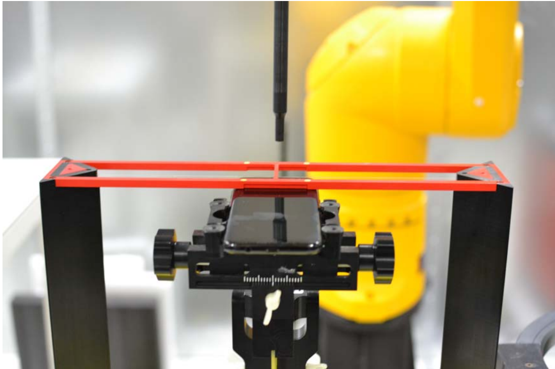
Figure 18-1 Ear Reference Point HAC Phantom Alignment
