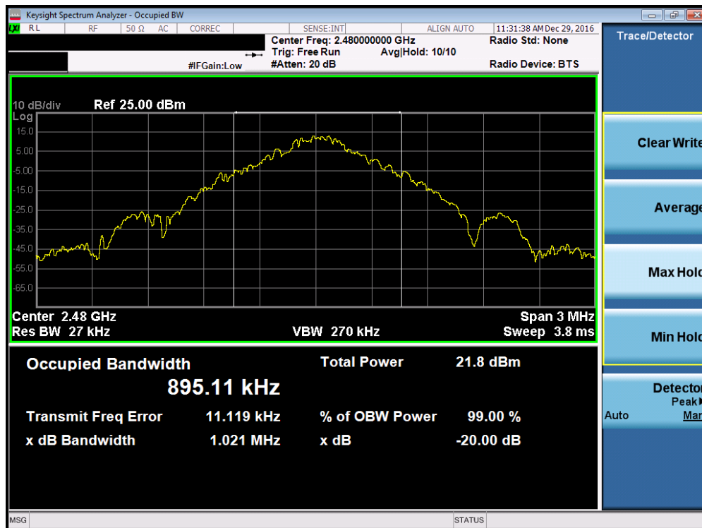
Plot 7-3. 20dB Bandwidth Plot (Bluetooth, 1Mbps – Ch. 78)
