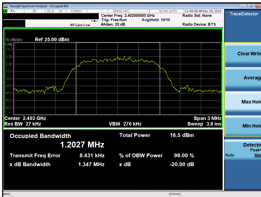
Plot 7-4. 20dB Bandwidth Plot (Bluetooth, 2Mbps – Ch. 0)
