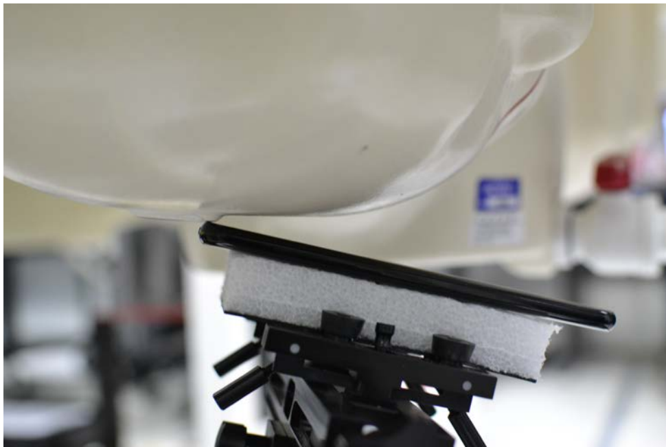
SAR Test Setup Photo 2 – Right Tilt
