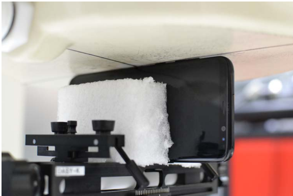
SAR Test Setup Photo 16 – Left Edge at 0 mm
