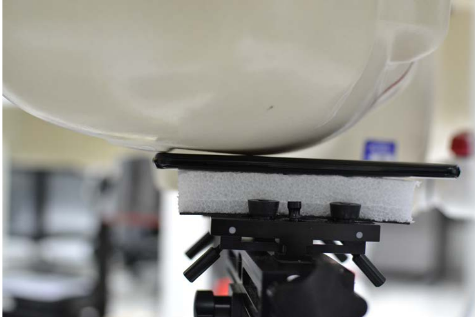
SAR Test Setup Photo 1 – Right Cheek
