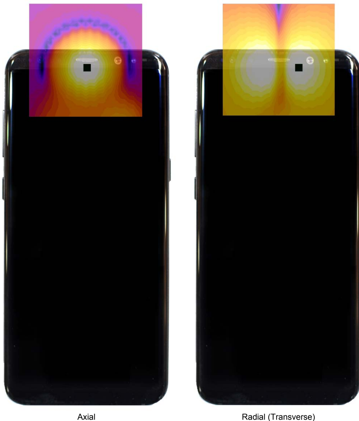
Figure 13-3 T-Coil Scan Overlay Magnetic Field Distributions
