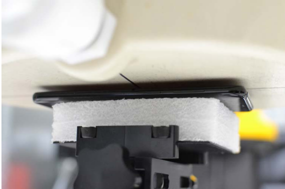
SAR Test Setup Photo 7 – Back Side at 5 mm
