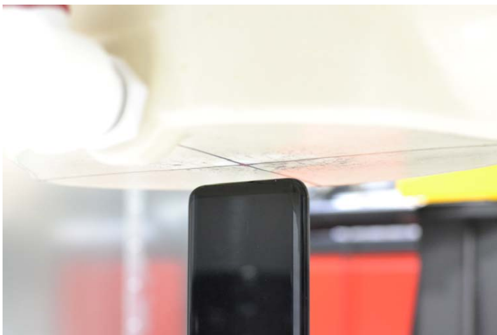
SAR Test Setup Photo 14 – Bottom Edge at 10 mm
