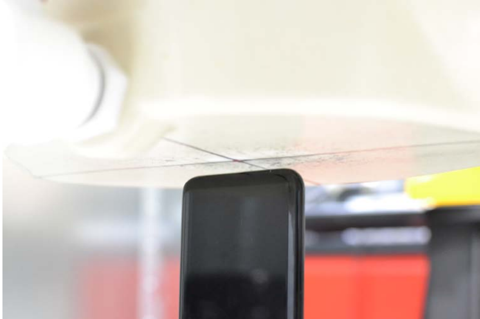
SAR Test Setup Photo 15 – Bottom Edge at 7 mm
