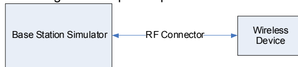
Figure 9-2 Power Measurement Setup
