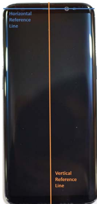
SAR Test Setup Photo 16 – Horizontal and Vertical Reference Lines
