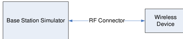
Figure 9-1 Power Measurement Setup
