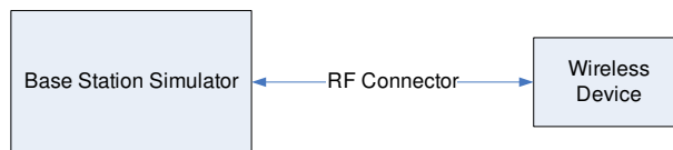
Figure 9-3 Power Measurement Setup
