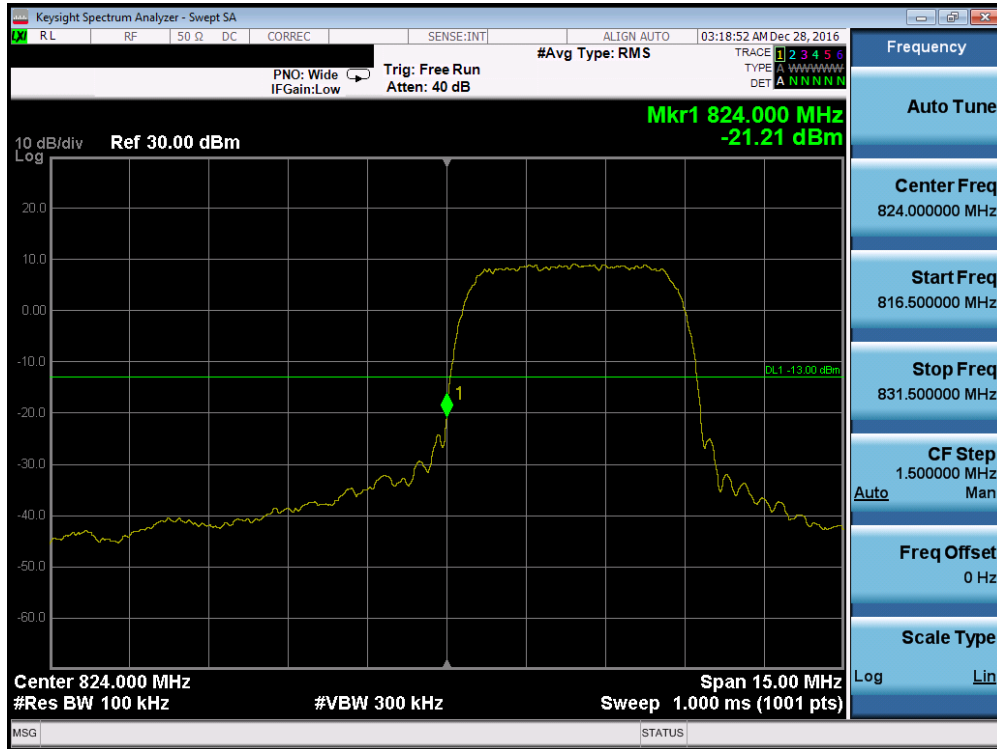
Plot 7-87. Band Edge Plot (Cellular WCDMA Mode – Ch. 4132)
