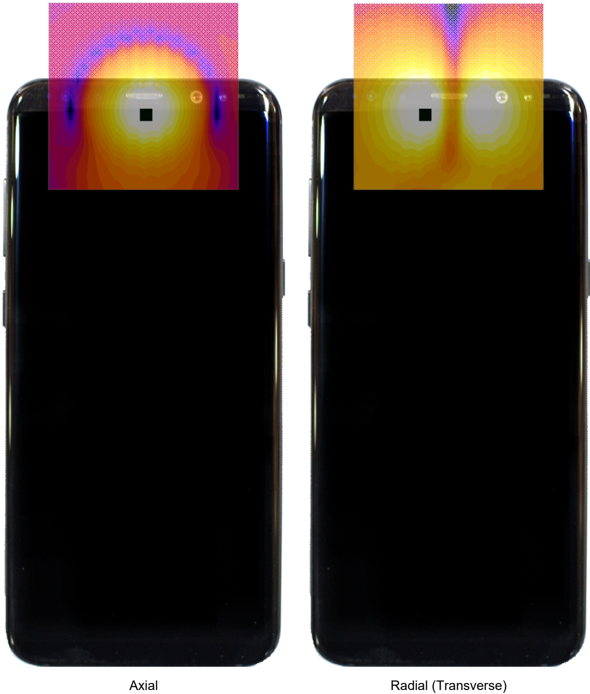
Figure 15-3 T-Coil Scan Overlay Magnetic Field Distributions
