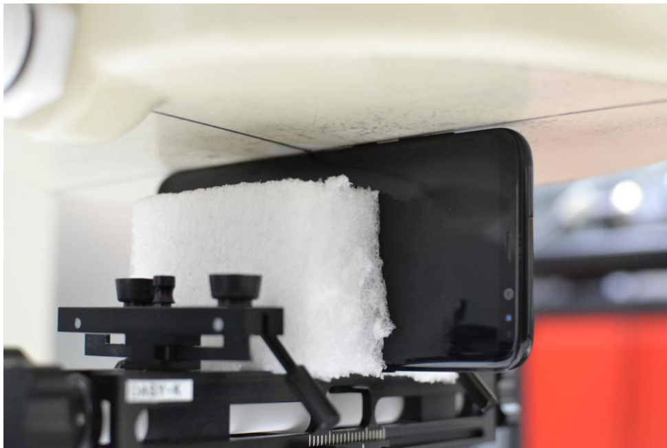
SAR Test Setup Photo 20 – Left Edge at 0 mm
