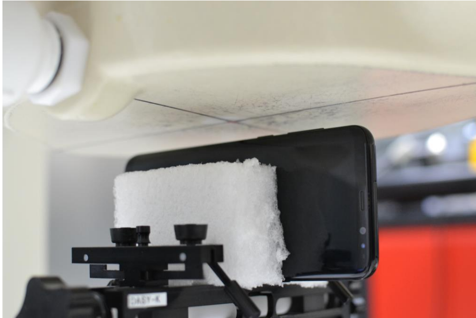
SAR Test Setup Photo 19 – Left Edge at 10 mm
