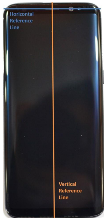
SAR Test Setup Photo 21 – Horizontal and Vertical Reference Lines
