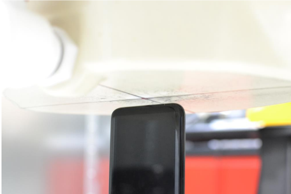
SAR Test Setup Photo 15 – Bottom Edge at 6 mm
