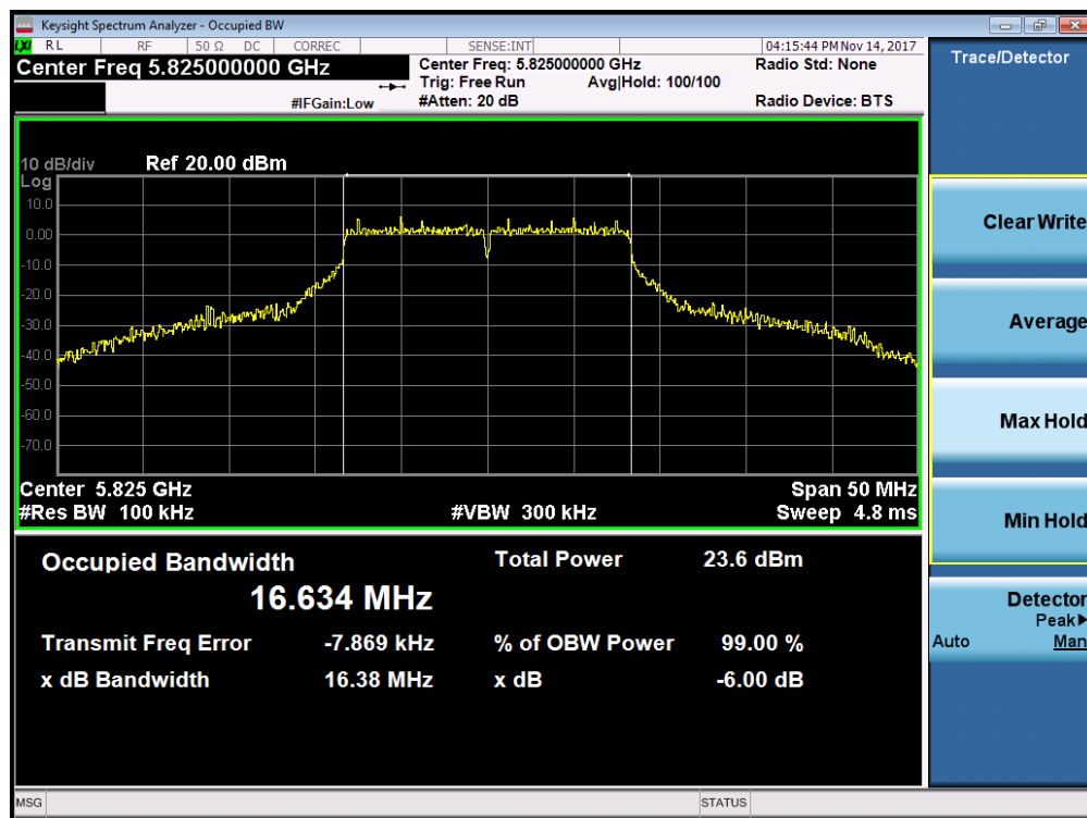
Plot 7-70. 6dB Bandwidth Plot (802.11a (UNII Band 3) – Ch. 165)
