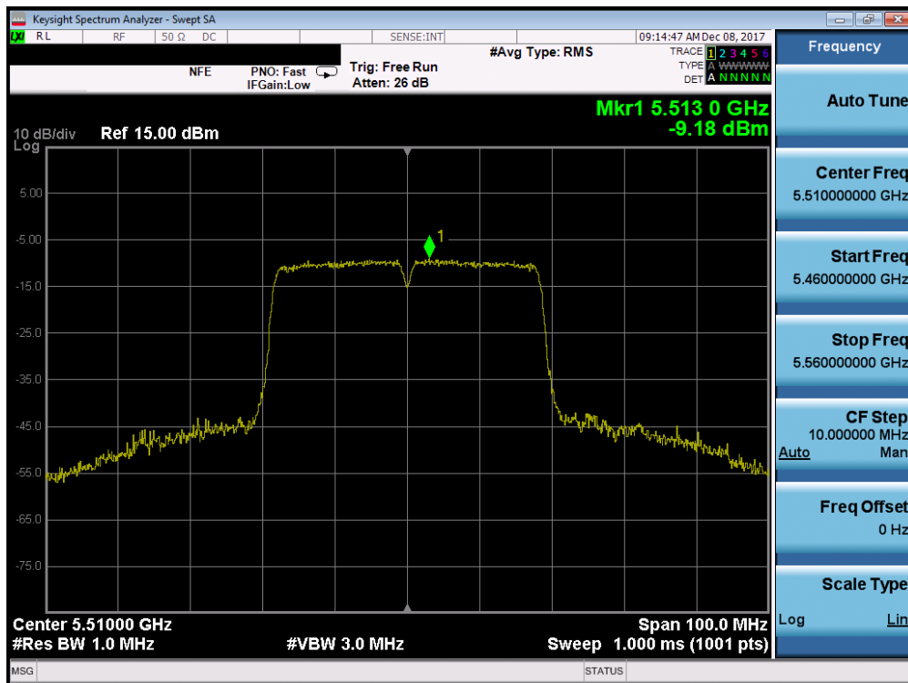
Plot 7-101. Power Spectral Density Plot (40MHz BW 802.11n (UNII Band 2C) – Ch. 102)
