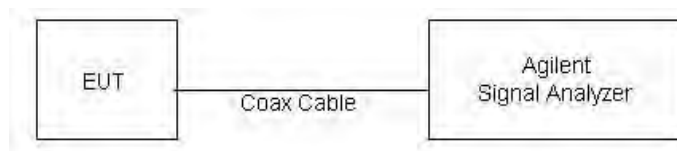
Figure 7-2. Test Instrument & Measurement Setup
