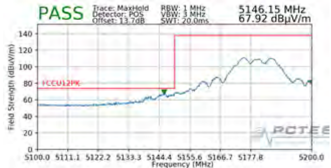
Plot 7-277. Radiated Lower Band Edge Plot (Peak – UNII Band 1)
