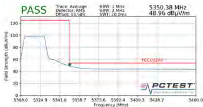
Plot 7-197. Radiated Upper Band Edge Plot (Average – UNII Band 2A)
