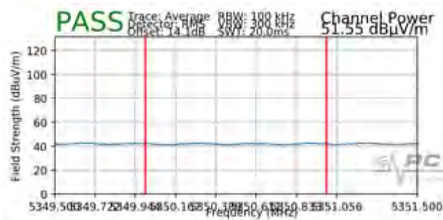
Plot 7-242. Radiated Upper Band Edge Plot (Average – UNII Band 2A)
