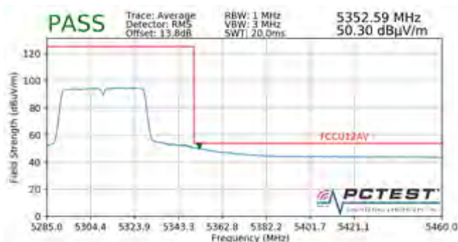
Plot 7-206. Radiated Upper Band Edge Plot (Average – UNII Band 2A)
