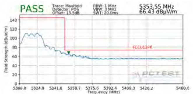
Plot 7-279. Radiated Upper Band Edge Plot (Peak – UNII Band 2A)
