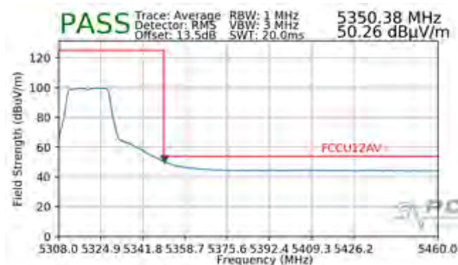
Plot 7-224. Radiated Upper Band Edge Plot (Average – UNII Band 2A)
