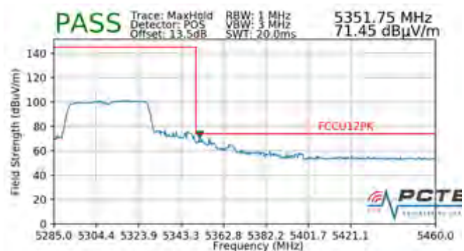
Plot 7-234. Radiated Upper Band Edge Plot (Peak – UNII Band 2A)
