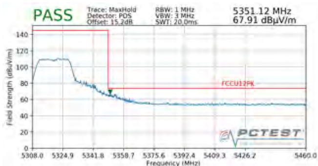
Plot 7-252. Radiated Upper Band Edge Plot (Peak – UNII Band 2A)
