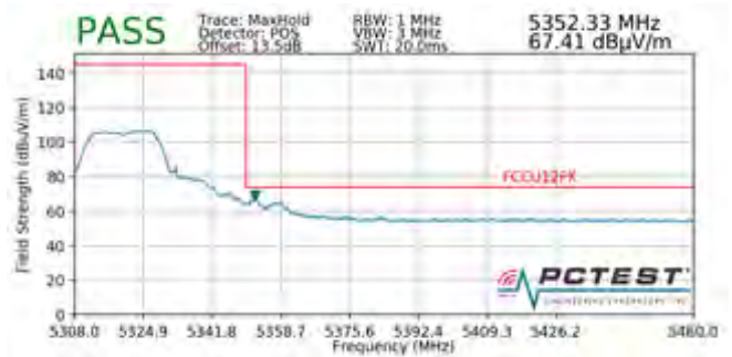
Plot 7-230. Radiated Band Edge Plot (Peak – WCP)
