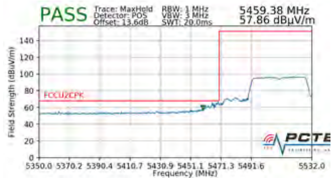
Plot 7-236. Radiated Lower Band Edge Plot (Peak – UNII Band 2C)
