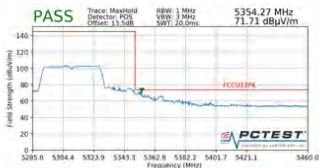
Plot 7-207. Radiated Upper Band Edge Plot (Peak – UNII Band 2A)
