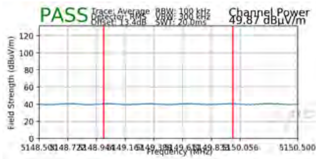
Plot 7-240. Radiated Lower Band Edge Plot (Average – UNII Band 1)
