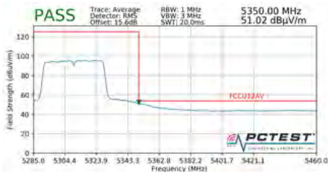
Plot 7-260. Radiated Upper Band Edge Plot (Average – UNII Band 2A)
