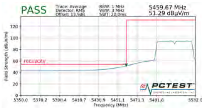
Plot 7-208. Radiated Lower Band Edge Plot (Average – UNII Band 2C)
