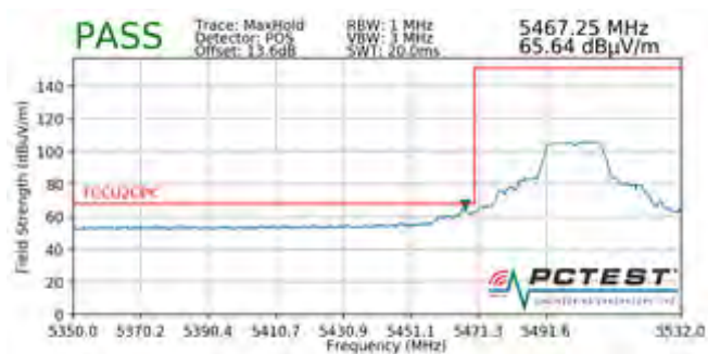
Plot 7-212. Radiated Band Edge Plot (Peak – WCP)
