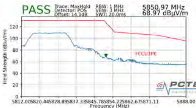
Plot 7-228. Radiated Upper Band Edge Plot (Peak – UNII Band 3)
