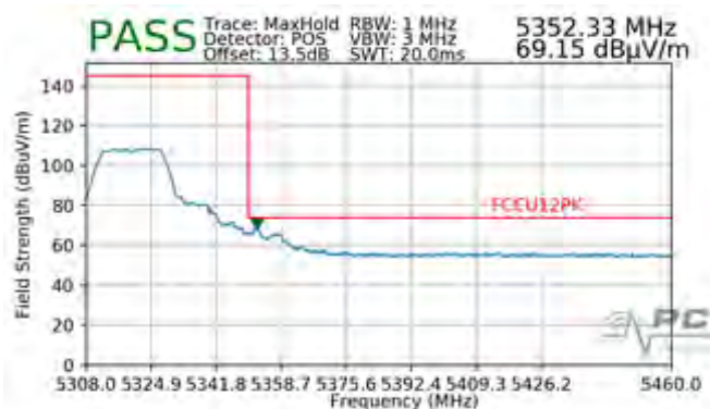
Plot 7-225. Radiated Upper Band Edge Plot (Peak – UNII Band 2A)
