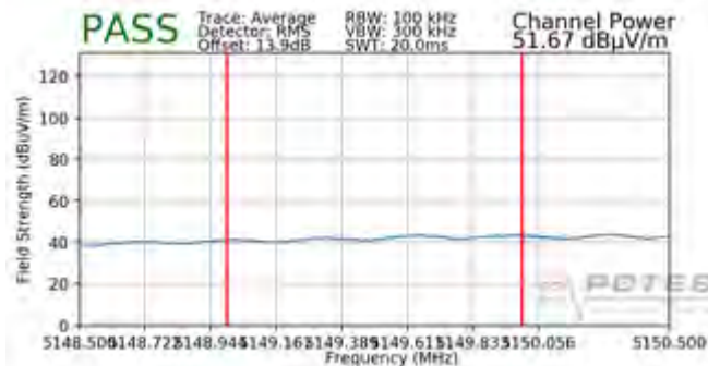
Plot 7-276. Radiated Lower Band Edge Plot (Average – UNII Band 1)
