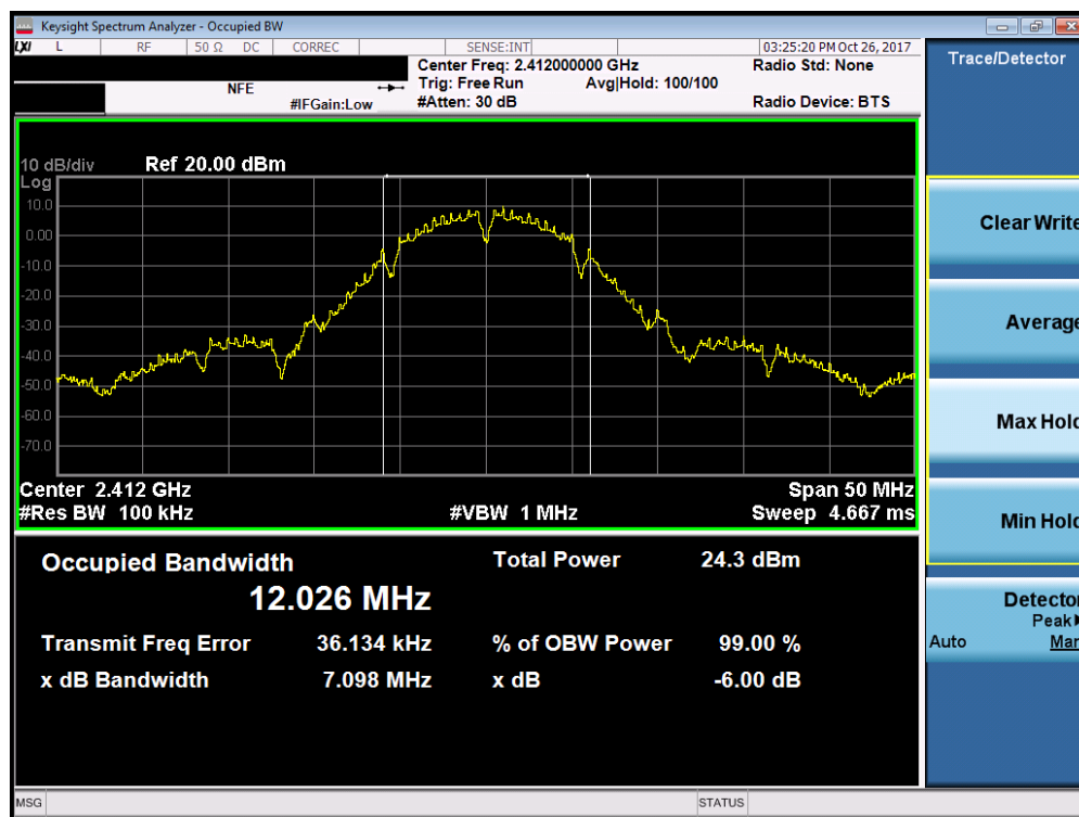
Plot 7-1. 6dB Bandwidth Plot (802.11b – Ch. 1)
