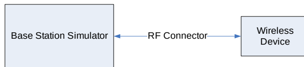
Figure 9-2 Power Measurement Setup
