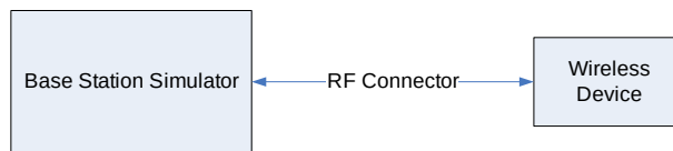
Figure 9-1 Power Measurement Setup
