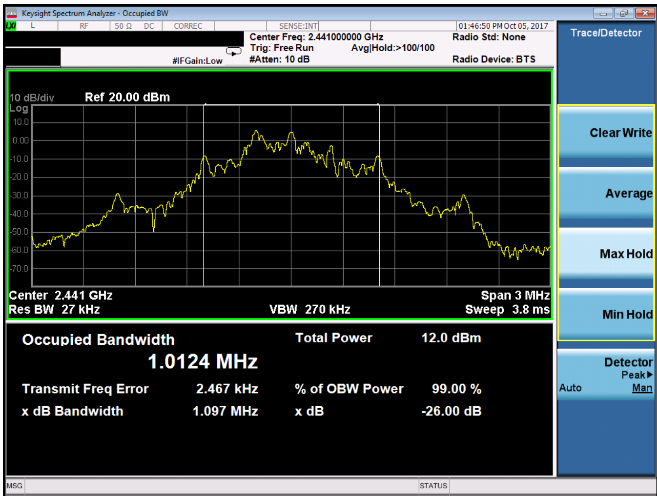
Plot 7-1. Occupied Bandwidth Plot (ANT+ – Ch. 39)
