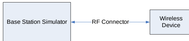
Figure 9-3 Power Measurement Setup
