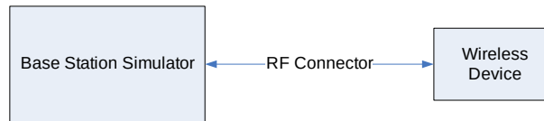
Figure 9-5 Power Measurement Setup
