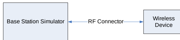
Figure 9-5 Power Measurement Setup
