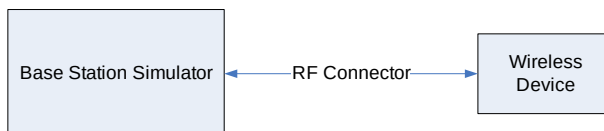
Figure 9-1 Power Measurement Setup
