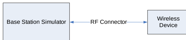
Figure 9-3 Power Measurement Setup
