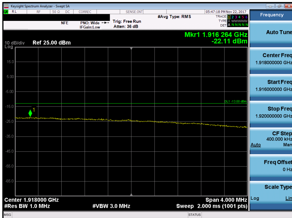
Plot 7-229. Upper Extended Band Edge Plot (Band 25 - 20.0MHz QPSK - Full RB Configuration)
