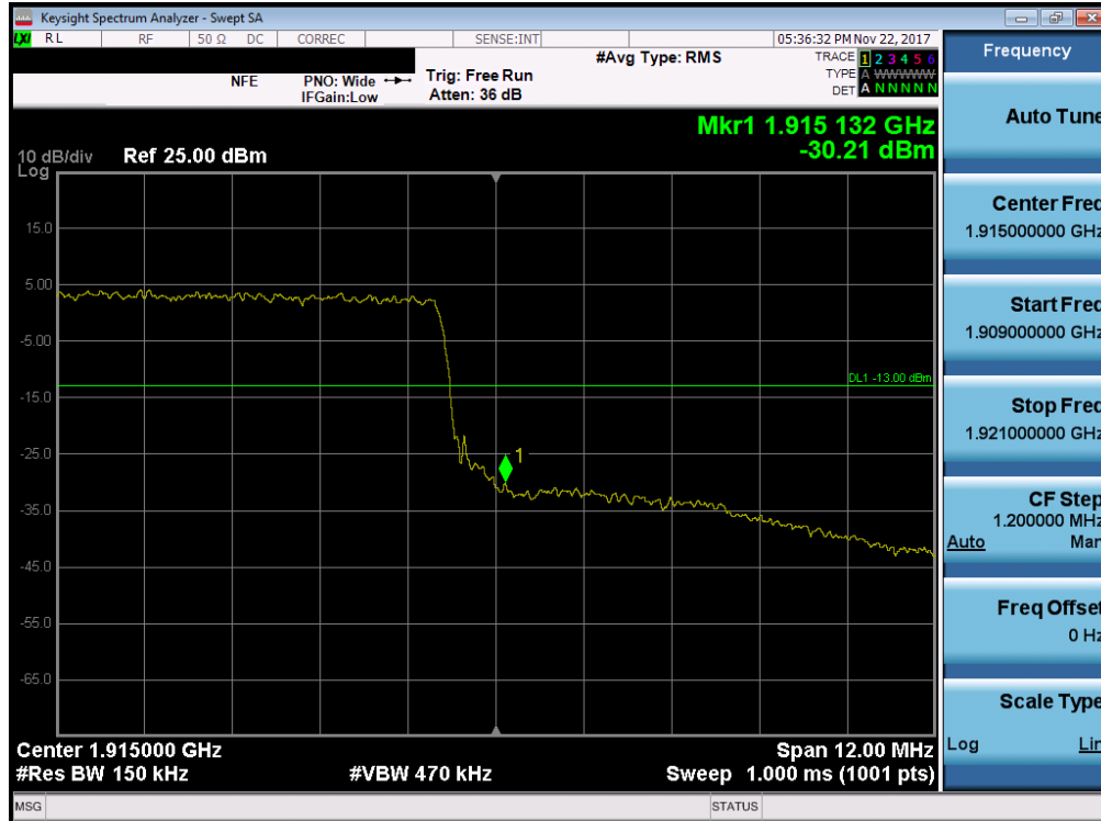
Plot 7-222. Upper Band Edge Plot (Band 25 - 15.0MHz QPSK - Full RB Configuration)
