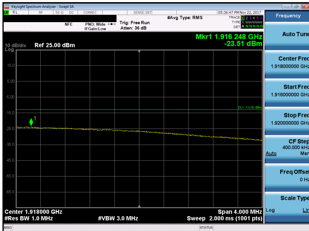
Plot 7-223. Upper Extended Band Edge Plot (Band 25 - 15.0MHz QPSK - Full RB Configuration)
