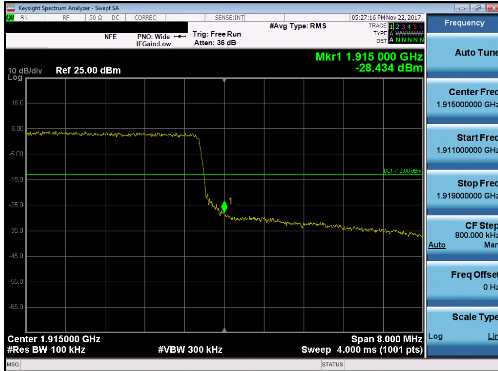
Plot 7-216. Upper Band Edge Plot (Band 25 - 10.0MHz QPSK - Full RB Configuration)
