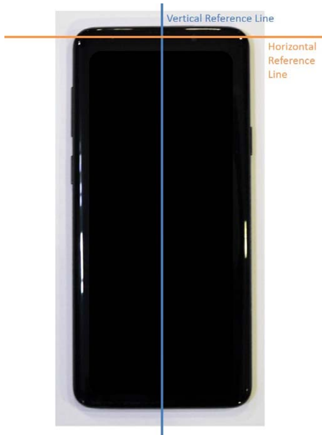
SAR Test Setup Photo 14 – Horizontal and Vertical Reference Lines
