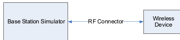
Figure 9-2 Power Measurement Setup
