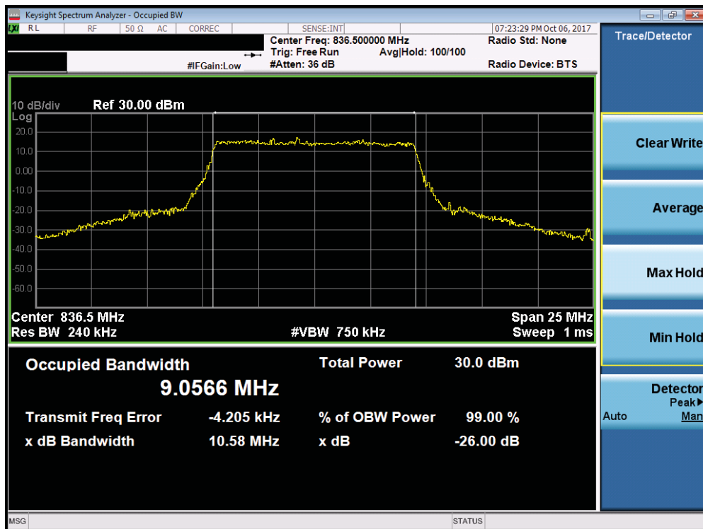
Plot 7-30. Occupied Bandwidth Plot (Band 5/26 – 10MHz 64-QAM - Full RB Configuration)
