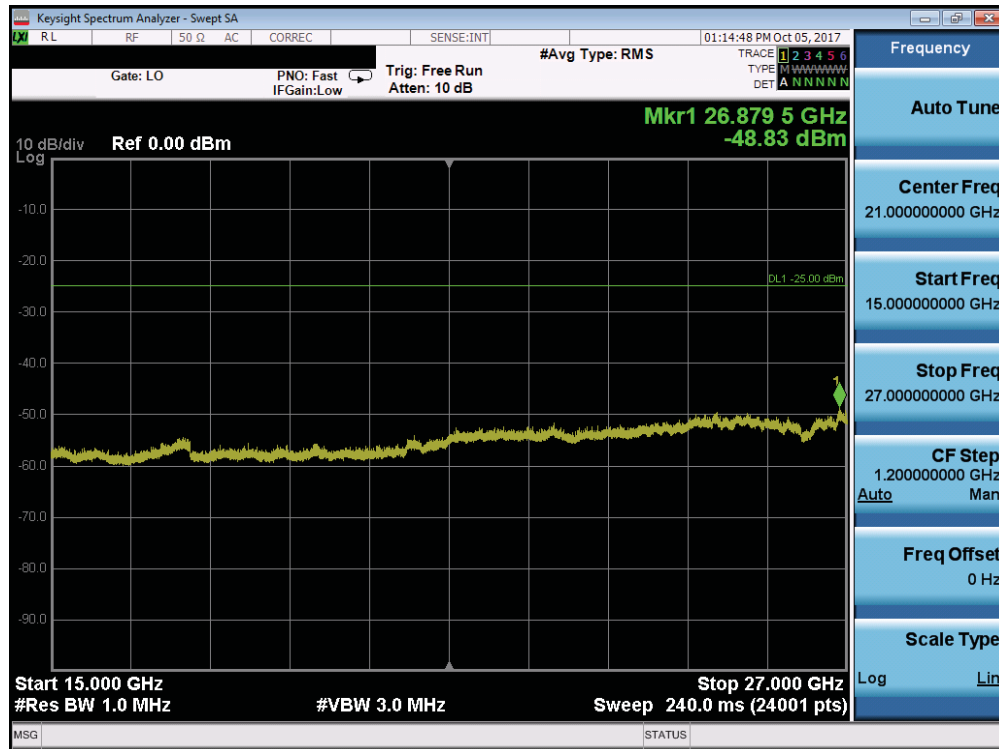
Plot 7-150. Conducted Spurious Plot (Band 38/41 - 10.0MHz QPSK - RB Size 1, RB Offset 0 - High Channel)
