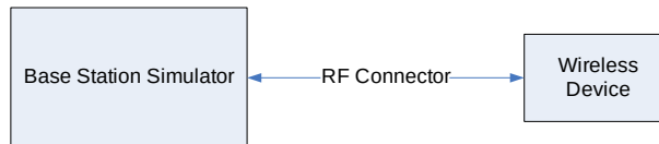
Figure 9-2 Power Measurement Setup
