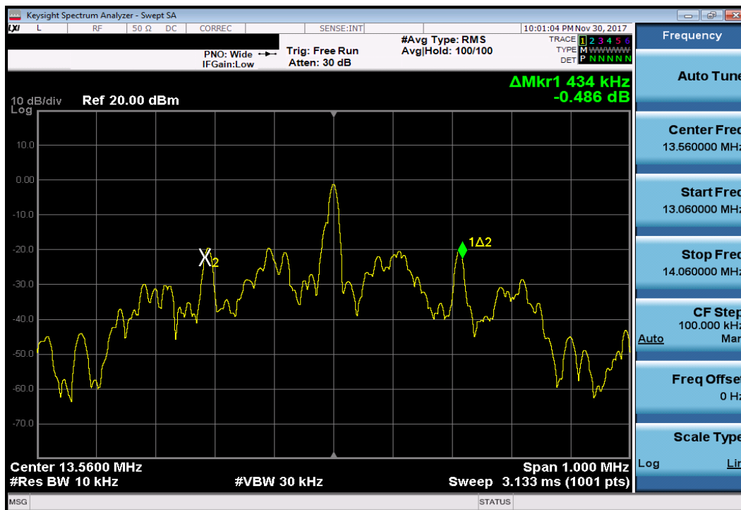
Figure 7-2. 20dB Bandwidth Plot
