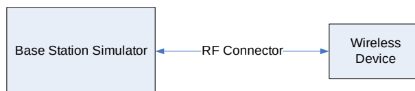
Figure 9-2 Power Measurement Setup
