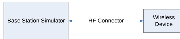
Figure 9-3 Power Measurement Setup
