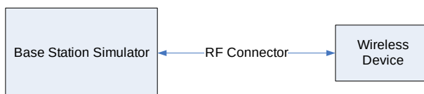
Figure 9-1 Power Measurement Setup
