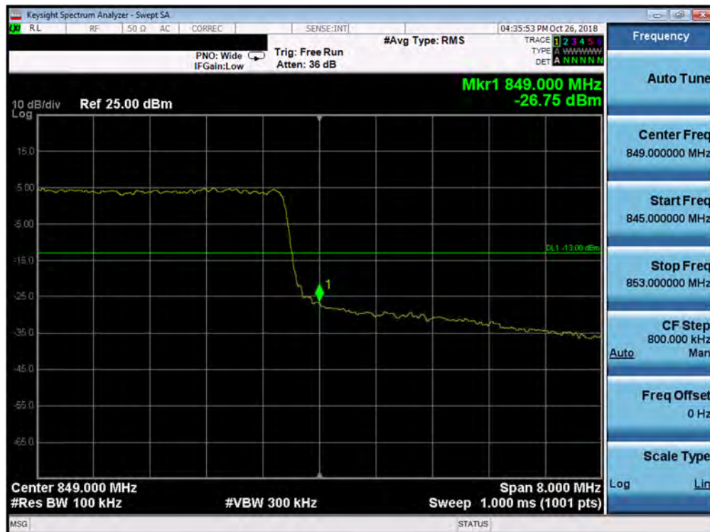
Plot 7-153. Upper Band Edge Plot (Band 26/5 - 10.0MHz QPSK - Full RB Configuration)
