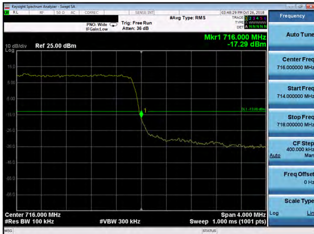
Plot 7-133. Upper Band Edge Plot (Band 12 - 3.0MHz QPSK - Full RB Configuration)
