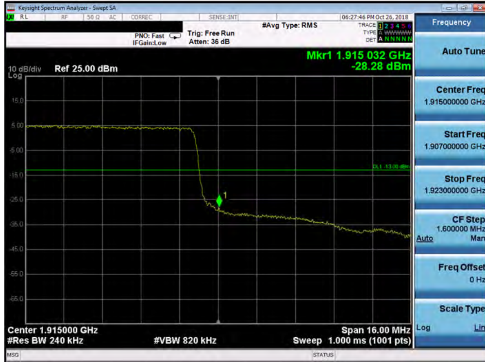
Plot 7-214. Upper Band Edge Plot (Band 25 - 20.0MHz QPSK - Full RB Configuration)
