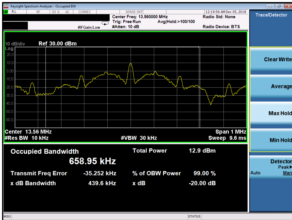
Figure 7-2. Occupied Bandwidth Plot
