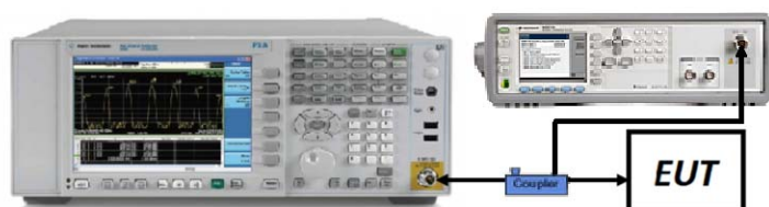
Figure 7-6. Test Instrument & Measurement Setup
