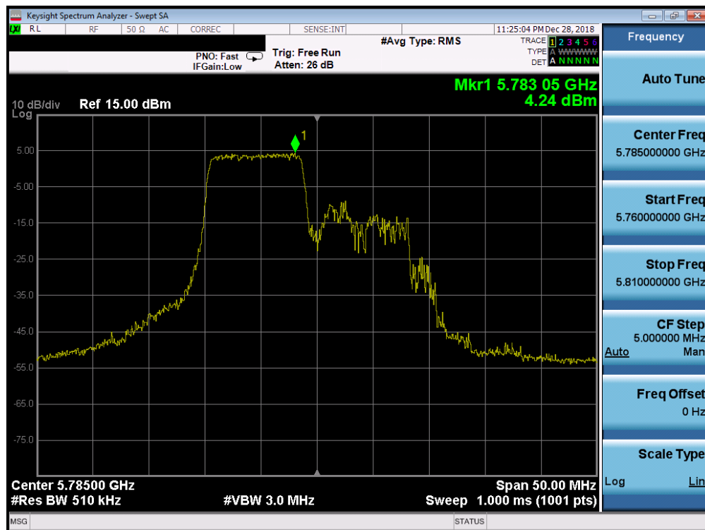
Plot 7-314. Power Spectral Density Plot SISO ANT2 (20MHz BW 802.11ax – 106 Tones (UNII Band 3) – Ch. 157)
