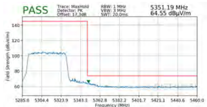
Plot 7-298. Radiated Upper Band Edge Plot SISO ANT1 (Peak – UNII Band 2A)
