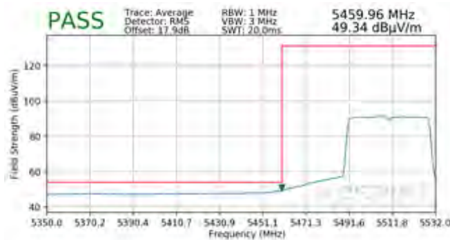
Plot 7-302. Radiated Band Edge Plot SISO ANT1 (Average - WCP)
