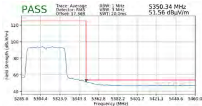
Plot 7-351. Radiated Upper Band Edge Plot MIMO (Average – UNII Band 2A)
