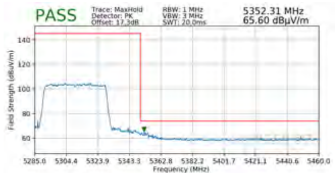
Plot 7-352. Radiated Upper Band Edge Plot MIMO (Peak – UNII Band 2A)
