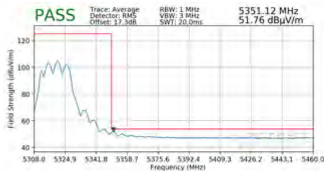
Plot 7-342. Radiated Upper Band Edge Plot CDD (Average – UNII Band 2A)
