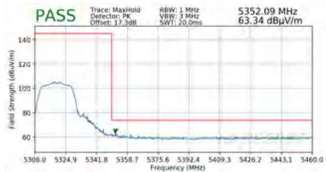
Plot 7-294. Radiated Band Edge Plot SISO ANT1 (Peak – WCP)
