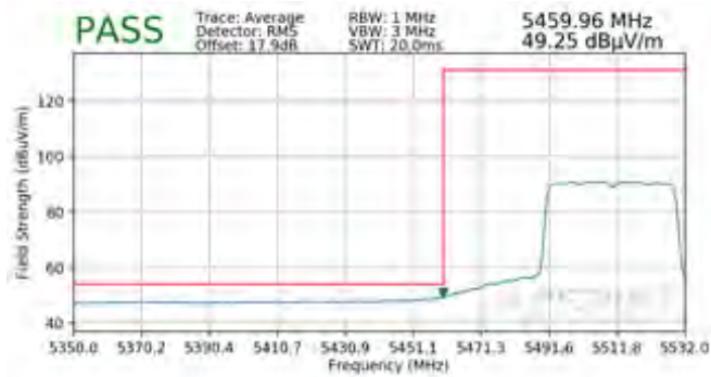
Plot 7-356. Radiated Band Edge Plot MIMO (Average – WCP)
