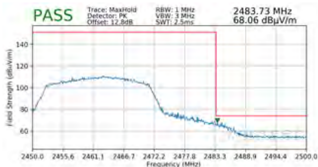
Plot 7-140. Radiated Restricted Upper Band Edge Measurement MIMO (Peak)
