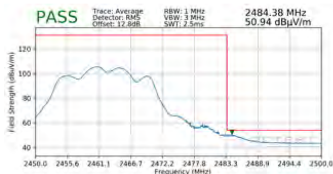
Plot 7-153. Radiated Restricted Upper Band Edge Measurement CDD (Average)
