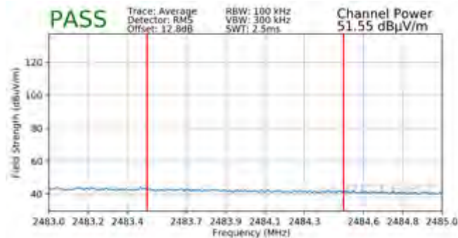
Plot 7-125. Radiated Restricted Upper Band Edge Measurement SISO ANT2 (Average)
