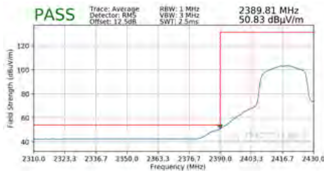
Plot 7-135. Radiated Restricted Lower Band Edge Measurement MIMO (Average)
