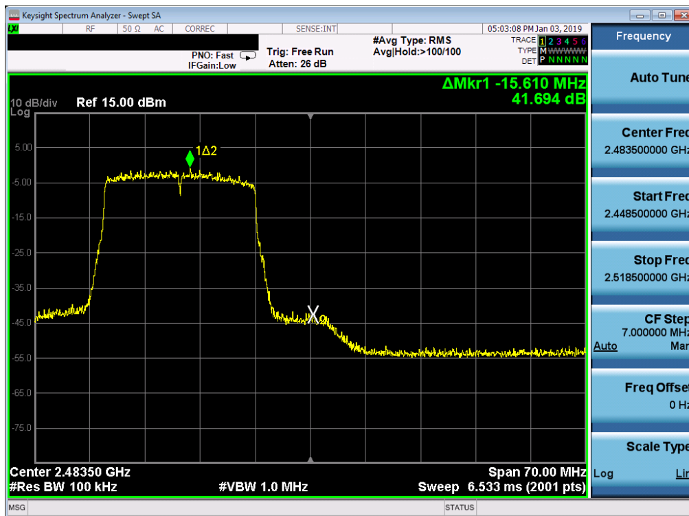
Plot 7-79. Band Edge Plot SISO ANT2 (802.11ax (2.4GHz) – Ch. 12)
