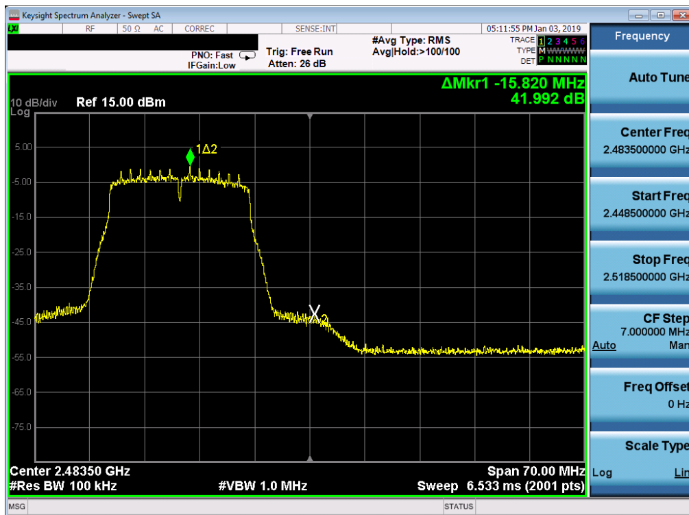
Plot 7-75. Band Edge Plot SISO ANT2 (802.11n (2.4GHz) – Ch. 11)
