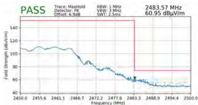
Plot 7-152. Radiated Restricted Upper Band Edge Measurement CDD (Peak)
