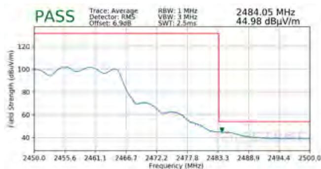
Plot 7-151. Radiated Restricted Upper Band Edge Measurement CDD (Average)
