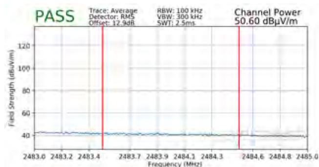
Plot 7-145. Radiated Restricted Band Edge Measurement MIMO with WCP (Average)
