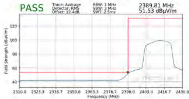
Plot 7-105. Radiated Restricted Lower Band Edge Measurement SISO ANT1 (Average)
