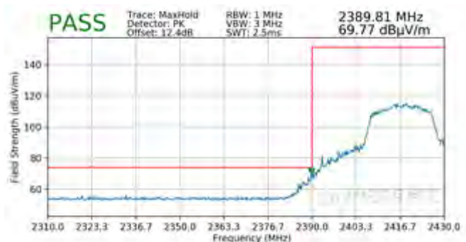
Plot 7-108. Radiated Restricted Lower Band Edge Measurement SISO ANT1 (Peak)
