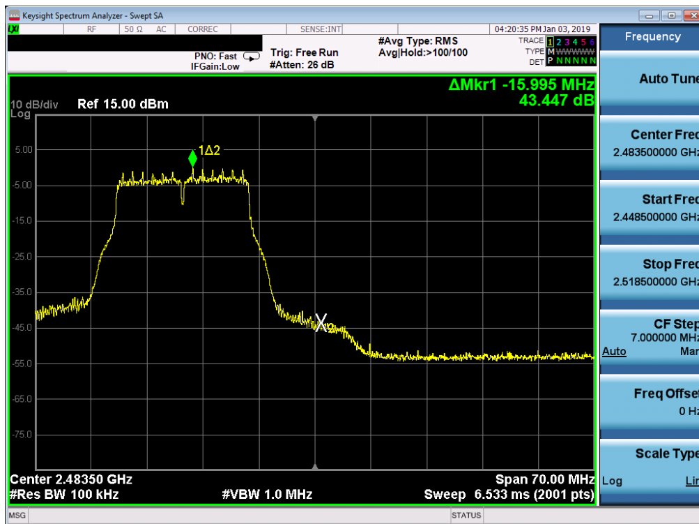
Plot 7-55. Band Edge Plot SISO ANT1 (802.11g – Ch. 12)
