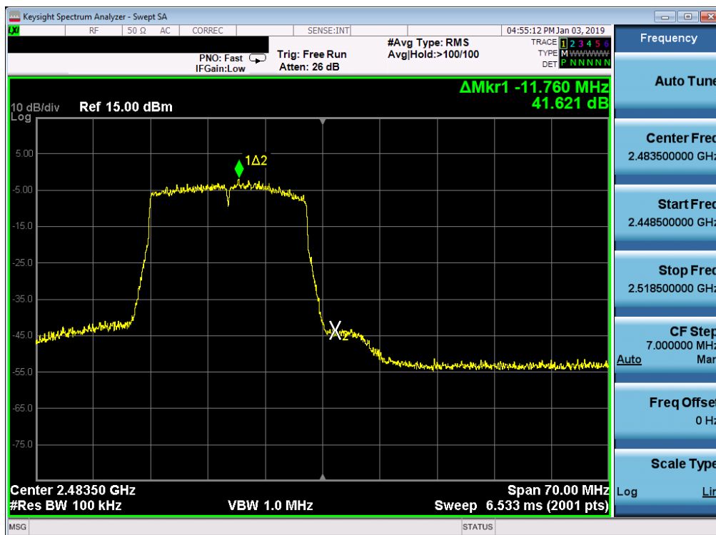
Plot 7-64. Band Edge Plot SISO ANT1 (802.11ax (2.4GHz) – Ch. 13)
