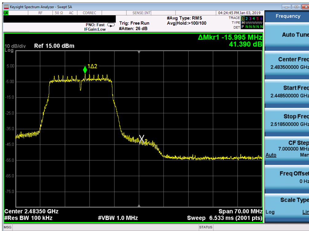
Plot 7-59. Band Edge Plot SISO ANT1 (802.11n (2.4GHz) – Ch. 12)
