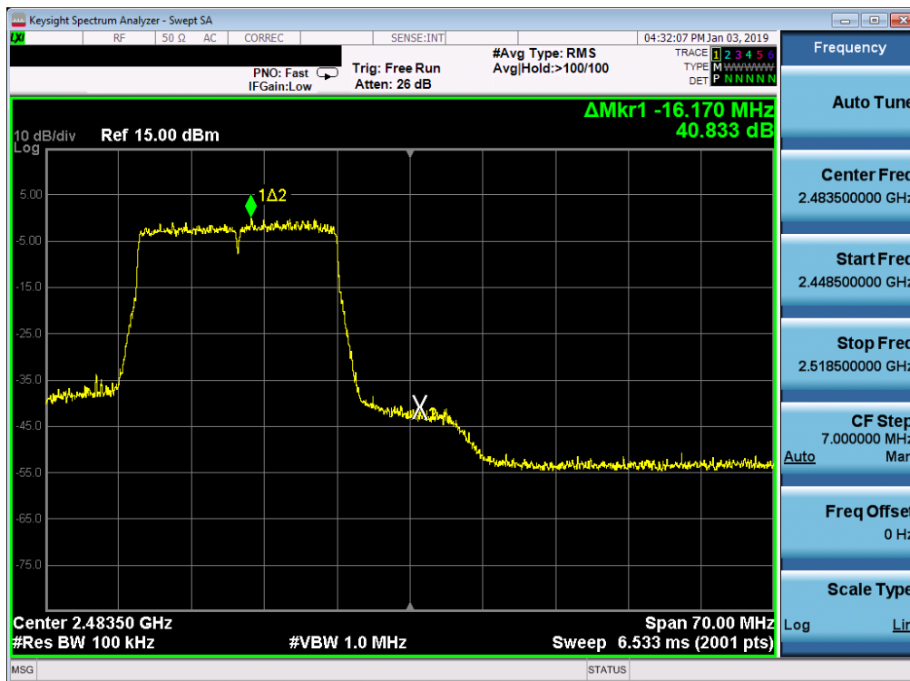
Plot 7-63. Band Edge Plot SISO ANT1 (802.11ax (2.4GHz) – Ch. 12)
