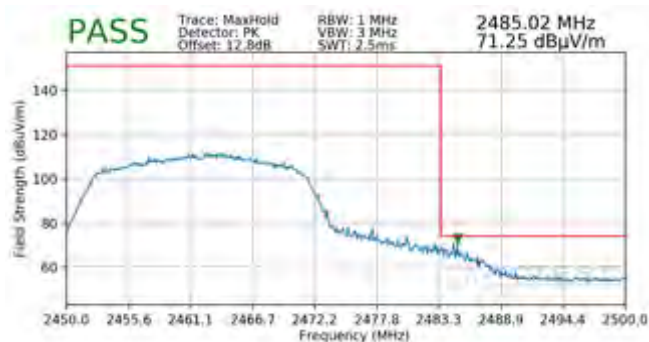
Plot 7-112. Radiated Restricted Upper Band Edge Measurement SISO ANT1 (Peak)
