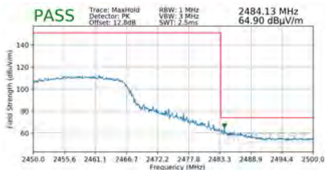
Plot 7-110. Radiated Restricted Upper Band Edge Measurement SISO ANT1 (Peak)
