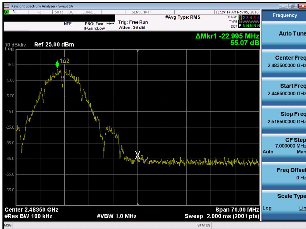
Plot 7-66. Band Edge Plot SISO ANT2 (802.11b – Ch. 11)
