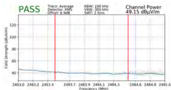
Plot 7-157. Radiated Restricted Upper Band Edge Measurement CDD (Average)
