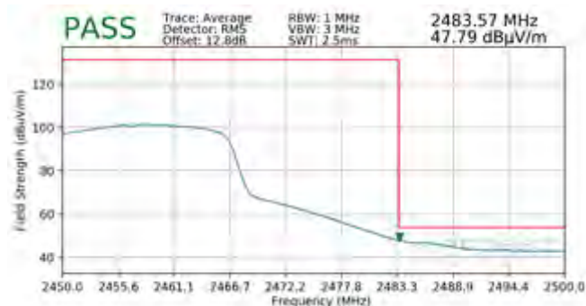
Plot 7-109. Radiated Restricted Upper Band Edge Measurement SISO ANT1 (Average)
