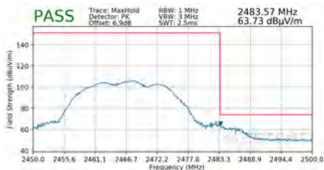
Plot 7-156. Radiated Restricted Upper Band Edge Measurement CDD (Peak)
