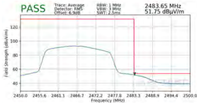
Plot 7-127. Radiated Restricted Upper Band Edge Measurement SISO ANT2 (Average)
