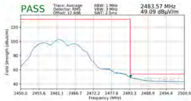
Plot 7-159. Radiated Restricted Band Edge Measurement MIMO with WCP (Average)
