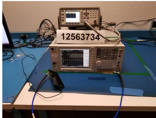
RF ANTENNA PORT CONDUCTED
