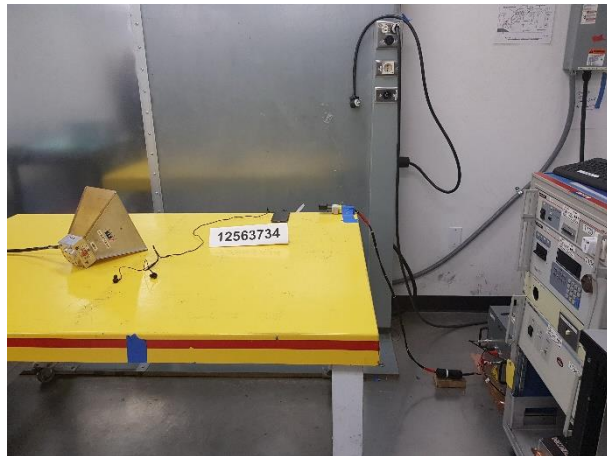
AC LINE CONDUCTED (FRONT)
