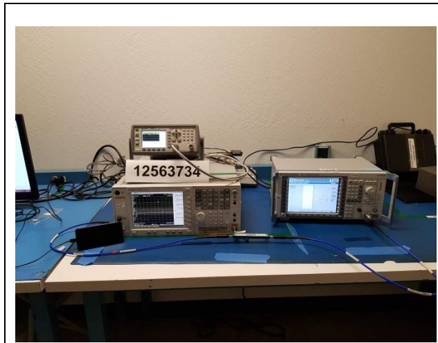
RF ANTENNA PORT CONDUCTED
