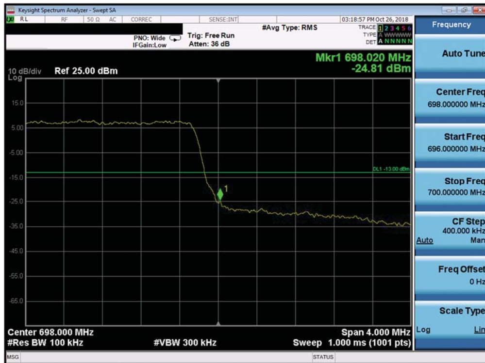
Plot 7-275. Upper Band Edge Plot (Band 71 - 5.0MHz QPSK - Full RB Configuration)
