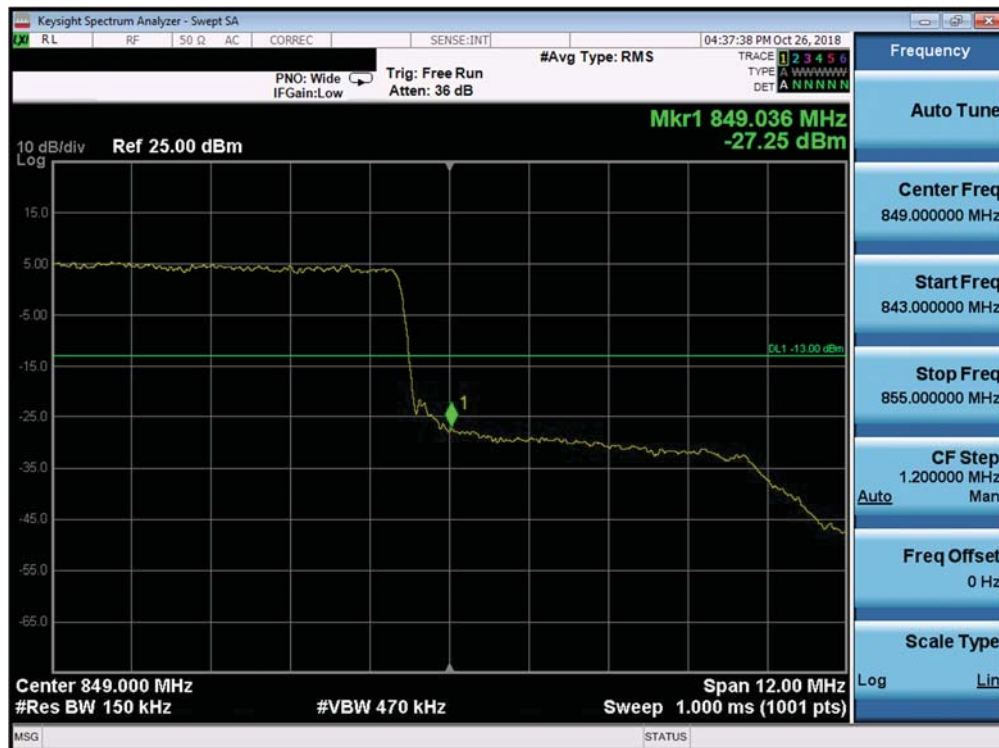
Plot 7-307. Upper Band Edge Plot (Band 26 - 15.0MHz QPSK - Full RB Configuration)
