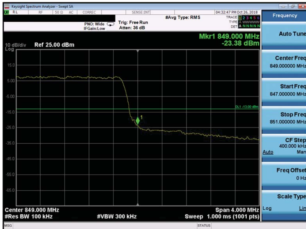
Plot 7-303. Upper Band Edge Plot (Band 26/5 - 5.0MHz QPSK - Full RB Configuration)
