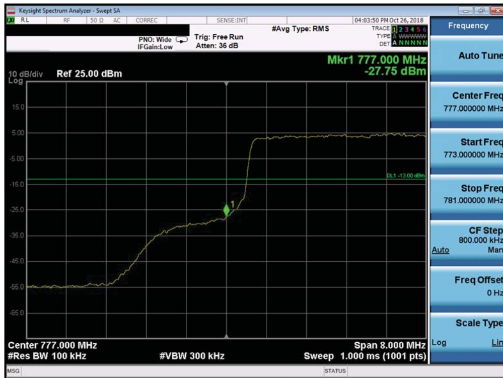
Plot 7-294. Lower Band Edge Plot (Band 13 - 10.0MHz QPSK - Full RB Configuration)
