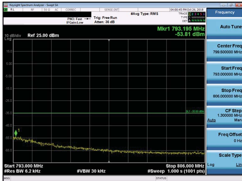
Plot 7-293. Upper Emission Mask Plot (Band 13 - 5.0MHz QPSK - Full RB Configuration)
