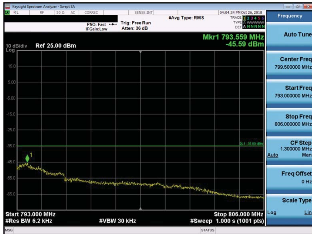
Plot 7-297. Upper Emission Mask Plot (Band 13 - 10.0MHz QPSK - Full RB Configuration)
