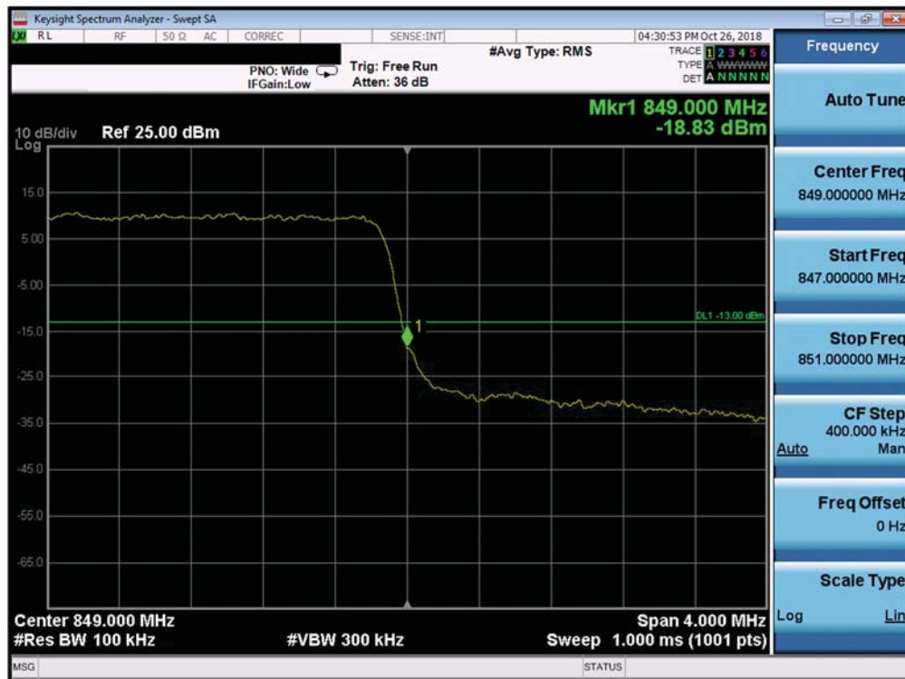
Plot 7-301. Upper Band Edge Plot (Band 26/5 - 3.0MHz QPSK - Full RB Configuration)
